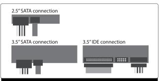
If you install hard drive on the mounting bracket, connect the necessary hard drive cable to device. If you install other card reader or device, please connect the cable using instruction from the device installation guide.
