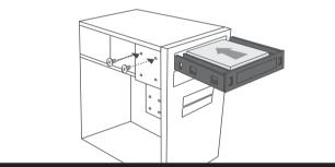
Slide the mounting bracket into the system chassis until the front panel is flush with the front of the case. Secure the 5.25" device using the provided screws on both side.
