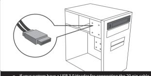
**8.** If your system have a USB 3.0 Header for connecting the 20 pin cable to use the front USB 3.0 port, please connect to the header. Some header may be on the motherboard or addon card.
