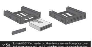
5a. To install 3.5 Card reader of other device, remove non-place or other and insert device into the 3.5" drive bay. Align the device front and secure using instruction from the device installation guide.
