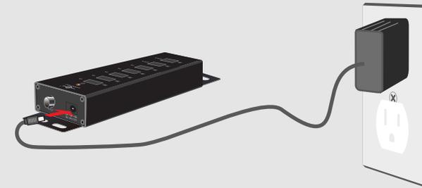
2. Connect the power adapter to the charging hub.
