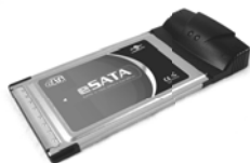
2-Port eSATA PCMCIA CardBus (UGT-ST350CB)
