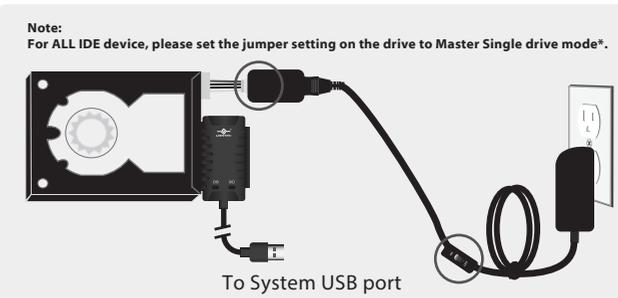
❖ 4b. Carefully connect the desired hard drive to the adapter.
