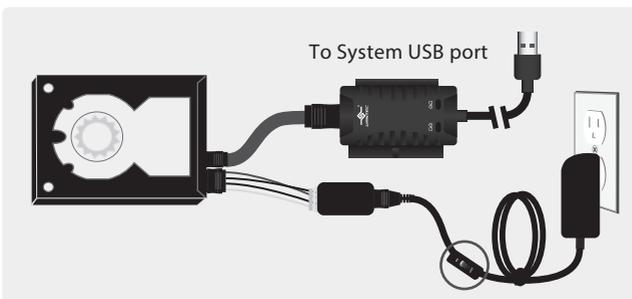
❖ 5. Once securely connected, you may switch ON the Adapter for device that need to power using AC Adapter. For 2.5" PATA(IDE) device you can skip this step. After Powering ON, wait 20 seconds before proceeding to the next step.
