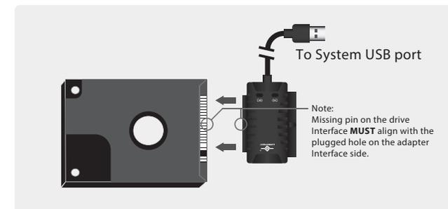
❖ 4c. Carefully connect the desired hard drive to the adapter. Proceed to step 6.
