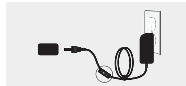
❖ 3. Note that there is an On/Off switch located along the AC power cable. Please make sure it is Off. (For 2.5" IDE, skip to Step 4c)
