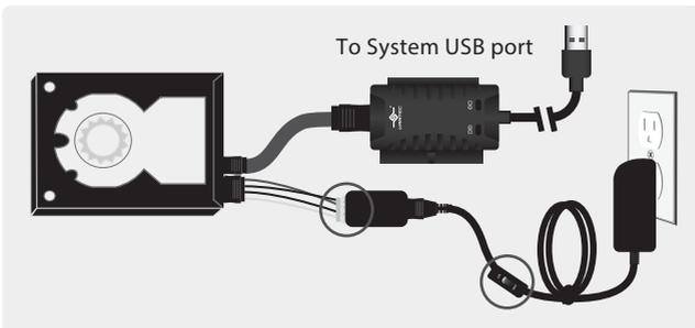
❖ 4a. Carefully connect the desired hard drive to the adapter.
