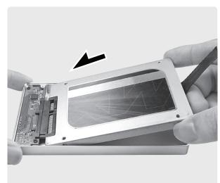
4. Slide the drive at an angle into the SATA interface until it is seated all the way into the interface and the drive seat into the enclosure. Keep the ribbon out.
