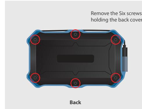
3. Turn to the back and remove the six screws holding the back cover.
