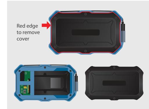
4. Pry along the red edge shown above to remove the back cover.
