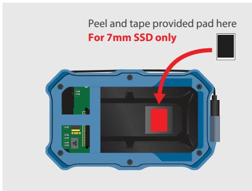
5. If you are using 7mm drive like a SSD, tape the provided pad shown above.
