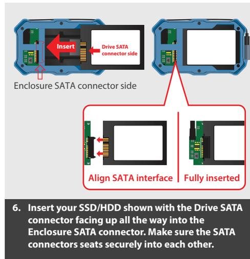
6. Insert your SSD/HDD shown with the Drive SATA connector facing up all the way into the Enclosure SATA connector. Make sure the SATA connectors seats securely into each other.
