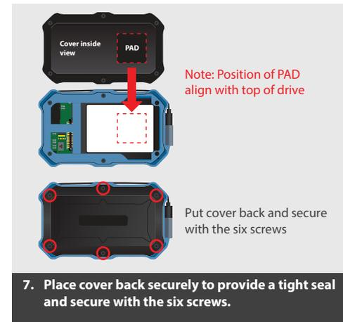
7. Place cover back securely to provide a tight seal and secure with the six screws.
