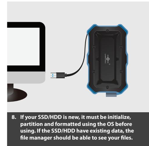
8. If your SSD/HDD is new, it must be initialize, partition and formatted using the OS before using. If the SSD/HDD have existing data, the file manager should be able to see your files.
