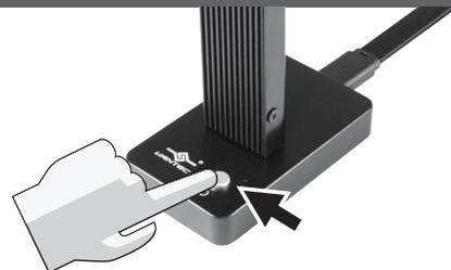
10. Press the power button to turn ON the DOCK and the LED should turn white (the WHITE LED indicates the DOCK is POWERED ON) the NVMe is ready for use.
