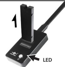
12. To safely remove the NVMe, please press the power button to turn OFF the DOCK before removing the NVMe module. The DOCK is OFF if you see the RED LED. If you did not see the RED LED, DO NOT REMOVE the NVMe module.
