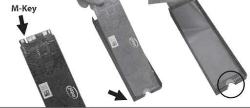
4. Align and set your NVMe module notch to the same side as the notch on the metal casing with the chip side facing the Thermal pad.
