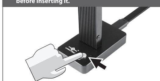
10. Press the power button to turn ON the DOCK and the LED should turn white (the WHITE LED indicates the DOCK is POWERED ON) the NVMe is ready for use.
