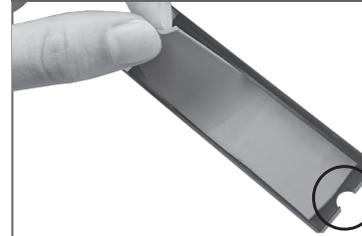
3. Use the THICK Thermal pad, peel off the protective film from one side and place it on the base metal casing without covering the notch as shown. Once it is in place remove the other protective film off the pad.
