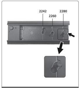
3. Note the length of your M.2 Module. This Dock will fit M.2 Module of size 2280, 2260, and 2242 in length. Adjust the Rubber Locking Mount to the right position for the length of your M.2 module by inserting it into the Rubber Mounting Hole and slide to lock the Rubber Locking Mount in place.
