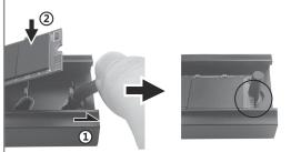
5. Insert your M.2 Module securely into the M.2 interface at an angle and push down while pushing the Rubber Locking Mount away slightly to let the M.2 module lock in place.
