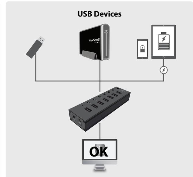
**3. Connect the USB 3.0 cable to the hub and computer.**
