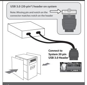
2b. Proceed to connect the USB 3.0 Header from this converted 5.25" Card Reader to your System motherboard or expansion card USB 3.0 Header (20pin) interface.
