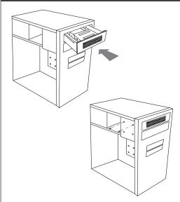
1b. Slide the front panel device into your case until the front panel is flush with the front of your case. Secure this converted 5.25" Card Reader device to your System Chassis with the provided screws.
