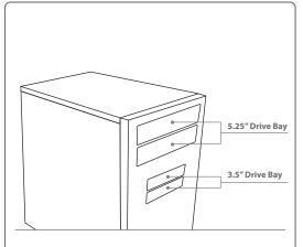
2. Locate an available 3.5" or 5.25" drive bay where you would like to install the device. If you are installing into a 3.5" Drive Bay, follow the steps listed below 1a and 2a.
