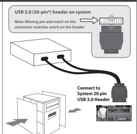
2a. Proceed to connect the USB 3.0 Header from this 3.5" Card Reader to your System motherboard or expansion card USB 3.0 Header (20pin) interface.
