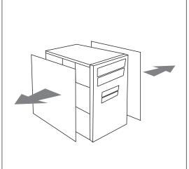
3. Prepare the System Chassis for installation by removing the System Chassis side panel(s) cover.
