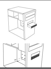
1a. Slide the front panel device into your case until the front panel is flush with the front of your case. Secure this 3.5" Card Reader device to your System Chassis with the provided screws.
