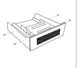
**2c.** Secure with the screws provided by the 3.5" to 5.25" front panel converter kit.
