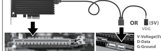
10. When installing this card into your system, make sure power is OFF and system power cord unplug from your wall outlet. Locate a free PCIe x4 or x8 or x16 expansion slot and insert this new PCIe card into the PCIe slot. Make sure the card is seated all the way into the slot and secure the card. Connect the other end of the ARGB cable using either 5V ARGB OR 5V VDG to the motherboard header.
