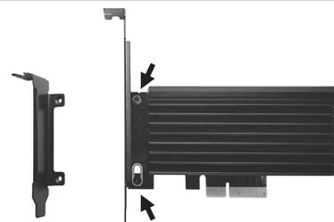
8. If your system is a low profile chassis and requires to replace the standard bracket to a Low Profile Bracket, remove the two screws holding the standard bracket and replace it with the provided Low Profile Bracket.
