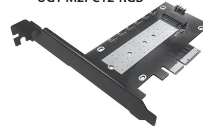
2. Before you unpack your NVMe module and take out the PCIe card, please be aware that these are sensitive devices and can be damaged by Static Electricity. Please ground yourself before handling them and hold it by the edge of the PCB and PCIe card.
