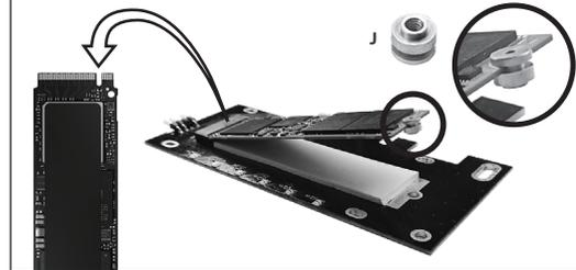
4. Align your M.2 Module with the M-Key interface to the RGB card M.2 connector, insert your NVMe module into the connector, put on the M.2 holding Nut (J) on your NVMe as shown.
