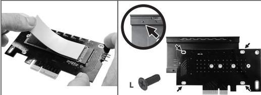
6. The Blue Thermal Pad comes in two thickness, (E) Thick Blue Thermal Pad, (F) Thin Blue Thermal Pad, please use the right pad according to the height of your M.2 SSD for proper Thermal Management. Select the right pad and apply the Blue Thermal Pad on top of your M.2 module.
