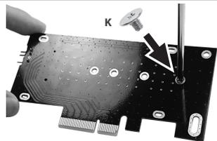
5. Push down and secure from the back of the card using Screw (K) onto the M.2 holding Nut (J) on Step #4.
