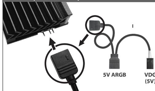
9. Connect the 3-pin ARGB cable (I) to the card. The other end of the ARGB cable connector is for the motherboard in the next installation step.
