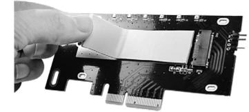
3. Remove the two plastic wrap on the Gray Thermal Pad and apply the pad on the heat transfer coating on the card.
