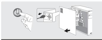
Turn off Computer System, unplug power and remove the cover of the Computer System
