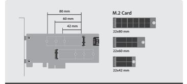
2. M.2 card comes in different length and size (42,60,80mm), match your M.2 card length to the hole alignment to decide which mounting hole to use.
