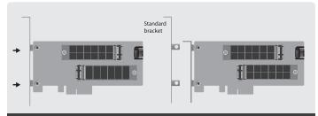
4. The card is ready to be integrated into your system. If you are adding this card into Slim or Low Profile System, please replace the standard bracket with a Low Profile Bracket provided. Remove the two screws holding the standard bracket and replace it with Low Profile Bracket and secure back the two screws hold the bracket.
