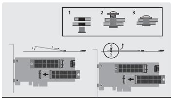
3. Attached M.2 Card by inserting the M.2 Card and secure using the washer and screw to hold the M.2 card in place.
