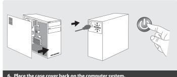
6. Place the case cover back on the computer system. Reattach the power to the Computer System and power ON the system.
