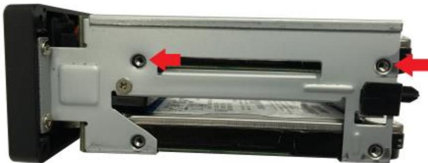
5. Secure both HDD/SSD with the 4 screws on each side of the Tray.
