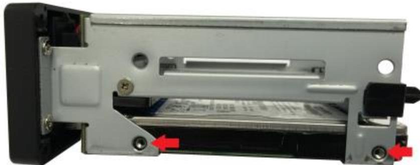
4. Insert the HDD/SSD into the top bay and push horizontally for both the SATA interface on the tray and drive to be fully inserted. The screw hole on the drive should align with the tray screw hole.
