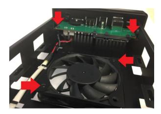
Remove the two screws holding the Printed Circuit Board first. Loosen the PCB and flip over to see the fan connector.
