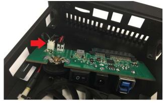
Turn over the Tray and remove the two screws holding the FAN.
